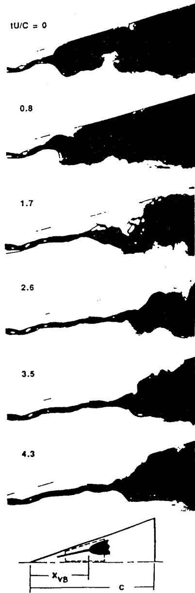
Fig. 11 Dye visualization of the effect of C_{\mu} = 0.036 on vortex breakdown on a 75-deg delta wing at \alpha = 54^\circ (Ref. 23).
